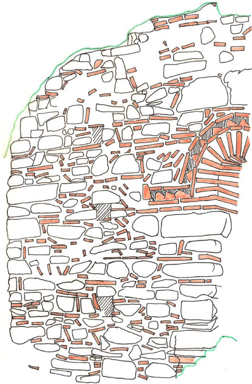
Fig. 70. Mt. Arakynthos, Panagia Trimitou, SW building. Drawing of a section of masonry on the E façade.
